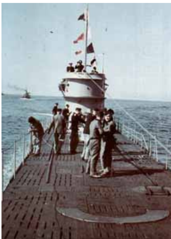
Above: The pristine looking Type IX U 128, with a Hellgrau 50 tower, in May 1941. The freshly-stained wooden deck looks dark, with only a tinge of brown showing through. The metal hatch on the right of the photo, and the C-shaped metal part at the bottom of the photo, have been painted black.
