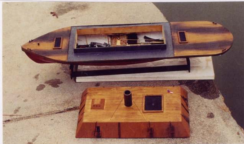
The hatch arrangement used on these "casemate" ships ensures a watertight seal.
