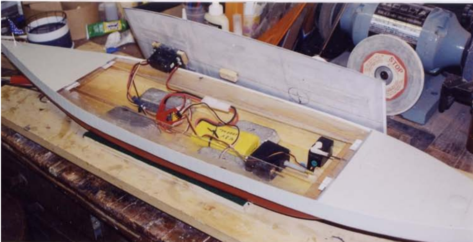
The roominess of the interior of the "block and sheet" construction hull shows up well here
