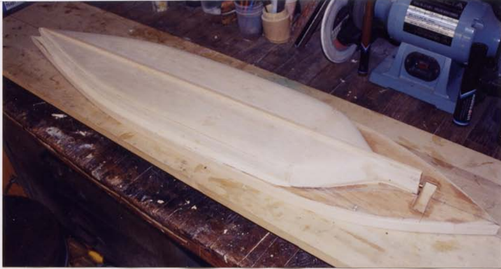
The roominess of the interior of the "block and sheet" construction hull shows up well here
