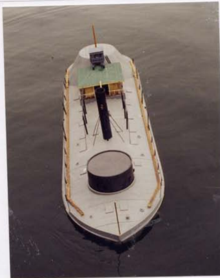
The humped "turtleback" deck was a means of providing internal space on the shallow draft river craft
