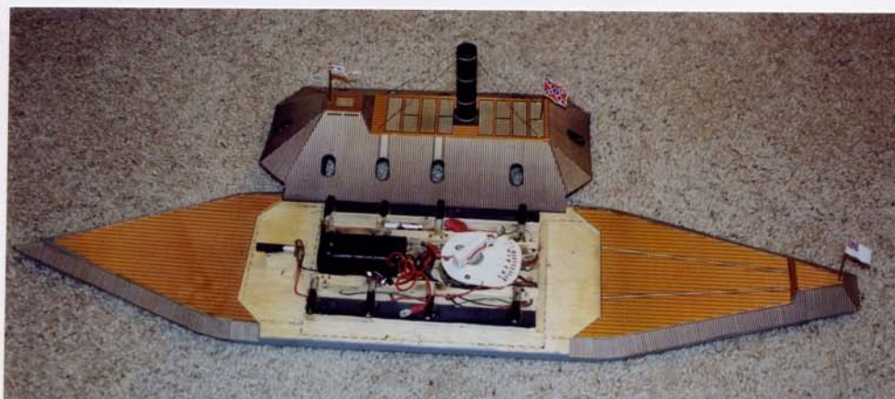
Interior layout showing timer, guns, and "raft" for hull.
