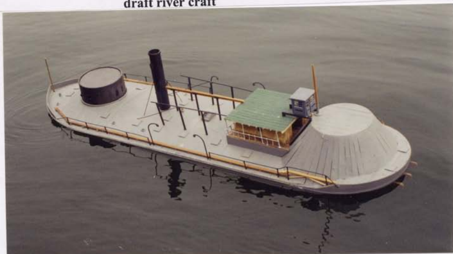
The humped "turtleback" deck was a means of providing internal space on the shallow draft river craft
