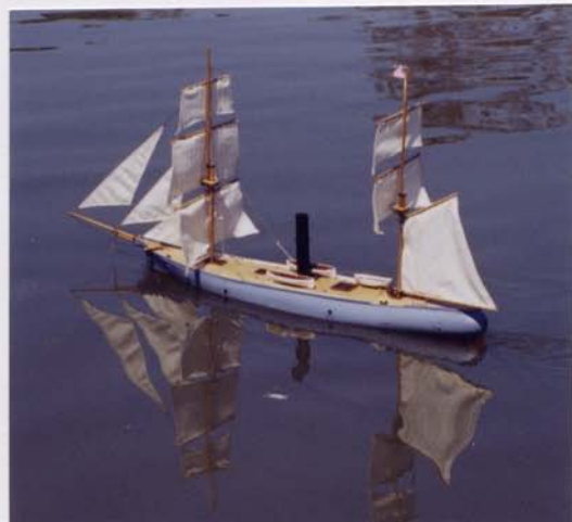
The Galena underway, using both sail and motor power. Note the reefed sails in the upper photo.
