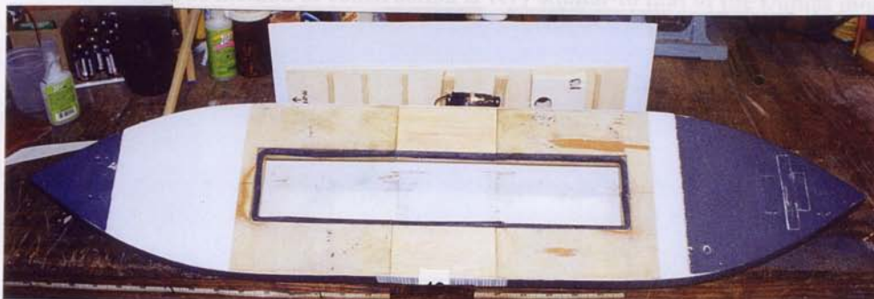
This view shows the 5 inch "stretch" added to the Dumas model.
