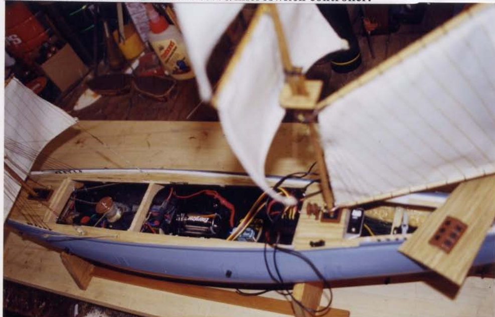
The interior is quite cramped, having to accommodate the usual R/C gear as well as two winches and their servo/microswitch controller.
