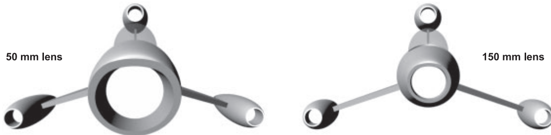
Figure 1.4.4. Perspective distortion can be drastically affected by distance to the camera and focal length of the lens.
